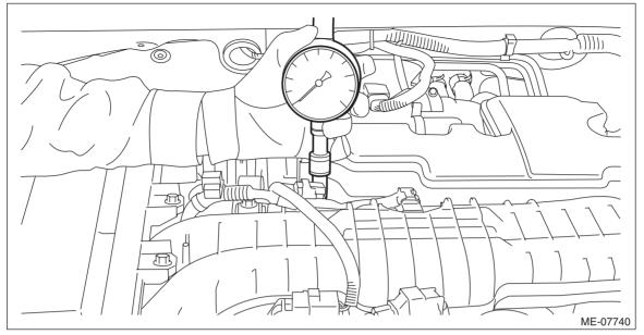
6) Keep the engine at idle speed and read the vacuum gauge indication.
