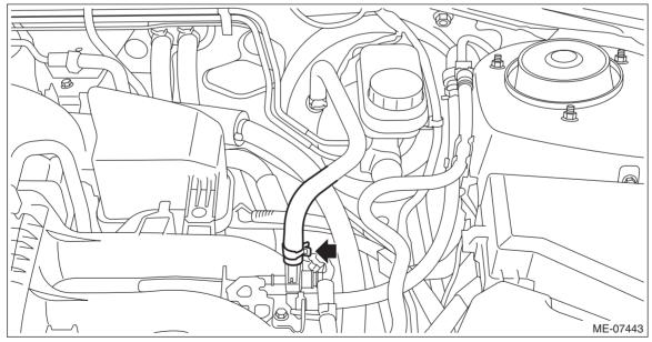
(2) Connect the vacuum gauge to the intake manifold.
